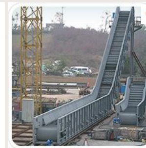
○ 보령화력 Dry-Type Bottom Ash System
