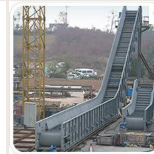
○ 보령화력 Dry-Type Bottom Ash System
