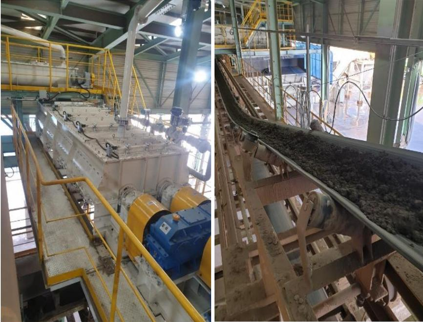
Last February, Samcheok Eco Materials completed the new installation of a pelletizer, which is a new mixing system used in the production line for fine aggregate.
