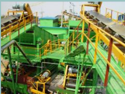
Facilities crushing and screening construction waste
