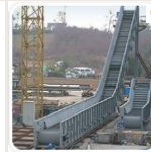
○ 보령화력 Dry-Type Bottom Ash System
