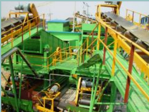
Facilities crushing and screening construction waste
